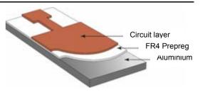
**ED COPPER** Thickness (μm) : 17,5 – 35 – 70 –105 - 210 **FR4 PREPREG** Thickness: 117 μm +/- 10%
